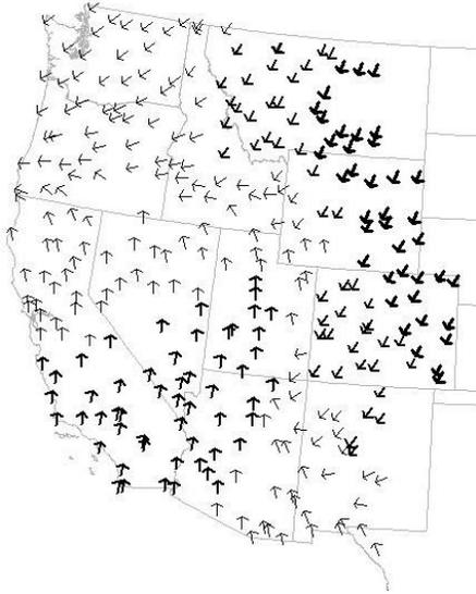
Figure 12: 0.473 Hz Mode Shape for 10K 26133 Gen Contingency
