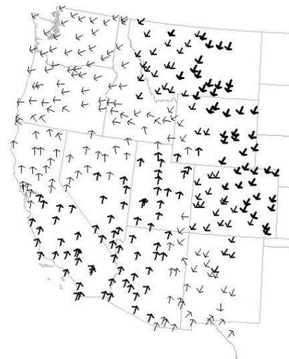
Figure 11: 0.474 Hz Mode Shape for 10K 40844 Gen Contingency
