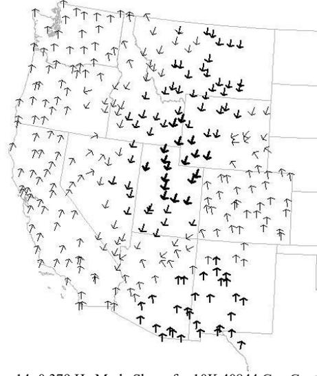
Figure 14: 0.379 Hz Mode Shape for 10K 40844 Gen Contingency
