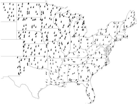
Figure 19: 0.264 Hz mode Shape for 70k 28344 Gen Contingency
