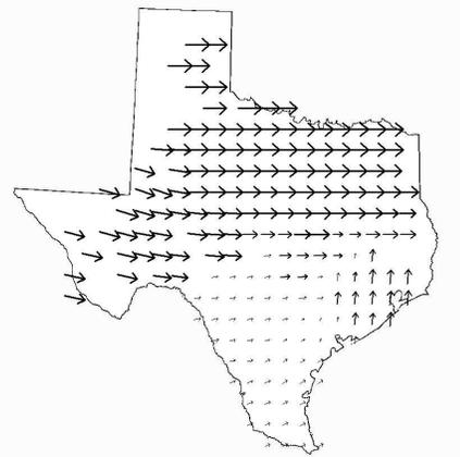
Figure 7: 0.552 Hz Mode Shape for 2K 7099 Gen Contingency
