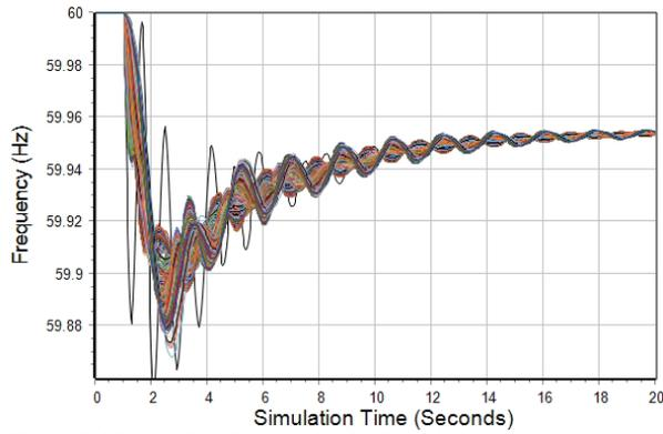
Figure 5: 2K Grid Bus Frequencies for Bus 7099 Gen Open Contingency
