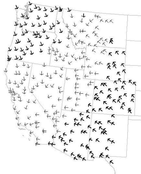
Figure 15: 0.373 Hz Mode Shape for 10K 26133 Gen Contingency
