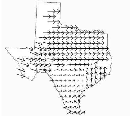
Figure 6: 0.531 Hz Mode Shape for 2K 5262 Gen Contingency
