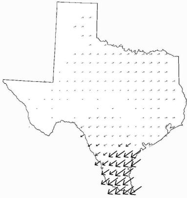
Figure 8: 0.625 Hz Mode Shape for 2K 5262 Gen Contingency
