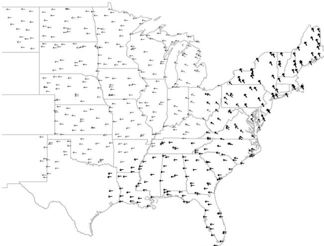
Figure 21: 0.209 Hz Mode Shape for 70K 38341 Gen Contingency
