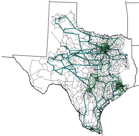
Fig. 2. Transmission lines of the synthetic Texas grid
