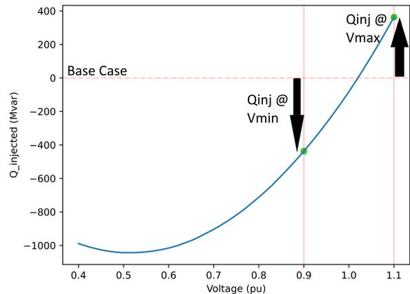
Fig. 1. QV curve for determining reserve requirements
